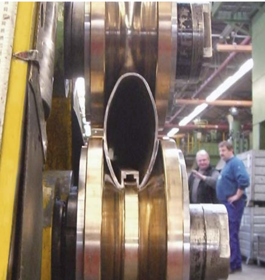
"The impossible is possible": BUTTING realizes your requirements for special geometric shapes
